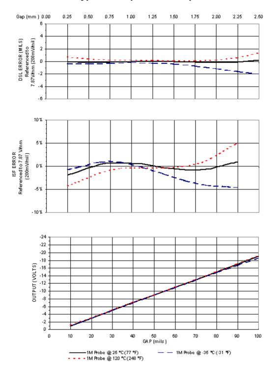
Figure 2 - 3300 5 metre XL Proximitor Sensor at high temperatures (3300 5mm probe and XL extension cable at 25° C)
