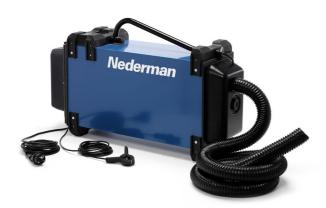
The Fume Eliminator (also called a Smoke Eater) is designed to be carried to the working area. Connected to a welding torch or to an extraction nozzle, the FE unit extracts the fume directly at source. FE 840 has a manual start/stop function while the FE 841 has an automatic start/stop function, which starts the unit as soon as the welding begins.
