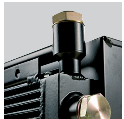
Temperature-controlled bypass valve Integrated Allows the oil to bypass the cooler matrix if the pressure drop is higher than 2,2 bar or less than the chosen temperature. The bypass closes when the oil temperature increases. Different closing temperatures available. Available for singlepass or two-pass matrix design
