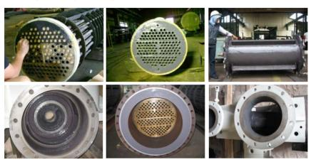
UPS 'Abrasion Resistant Ceramic Carbide Fluid' is a high performance fluid grade engineering resurfacing compound designed for use in fluid flow environments.
