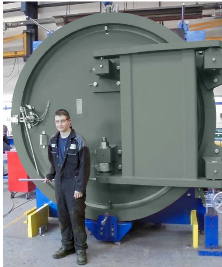
90" Horizontal Bandlock™2 Closure (90 barg) as supplied into the Middle East
