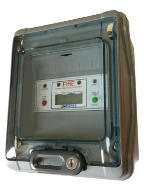
The Digital Location Interface (DLI) monitors the Linear Heat Detection (LHD) cable and when activated identifies the location of the alarm. The distance in meters is then displayed on the 4 digit LCD. Providing detection and location along the complete length of the LHD cable.
