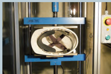
V-Gard 500 tested for lateral deformation
